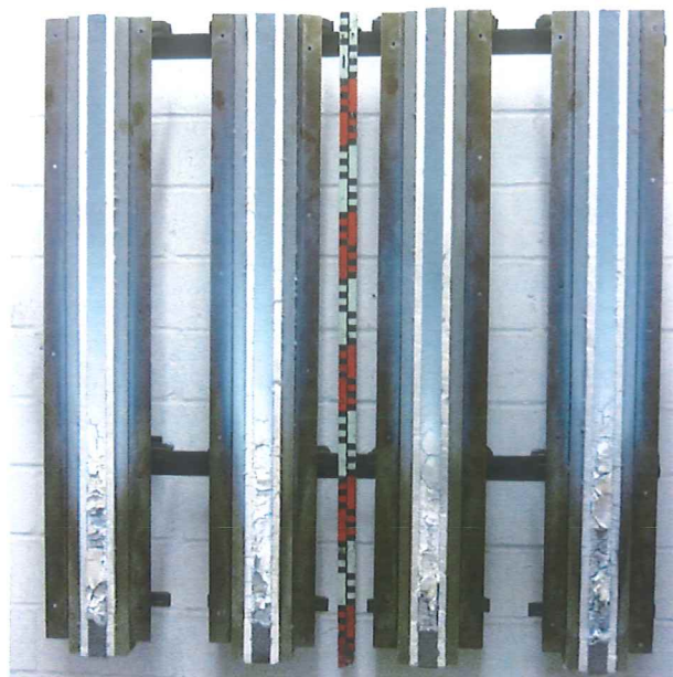
figure 4: appearance of the specimen B after 10-minutes burning
