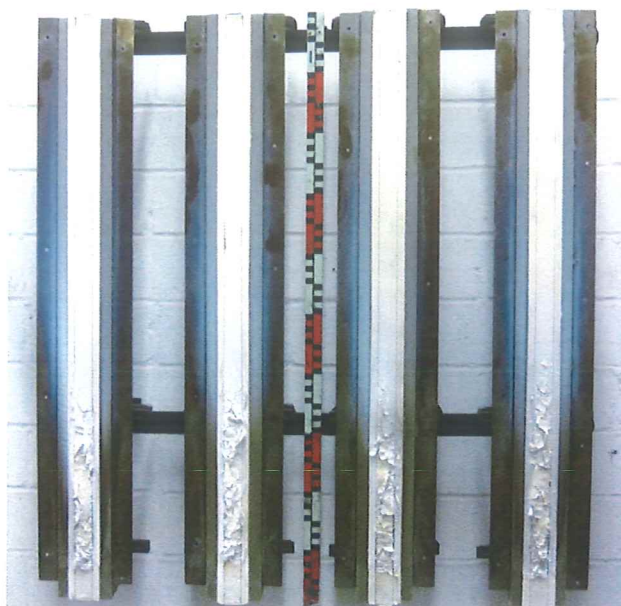
figure 3: appearance of the specimen A after 10-minutes burning
